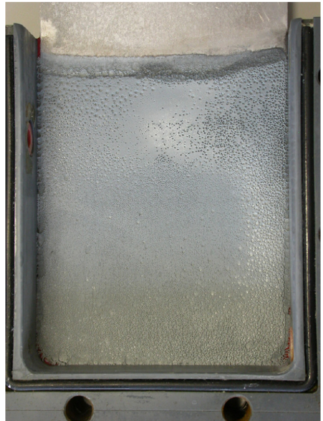
Fig. 13. Aspect of the zinc coated cathode at the end of experiment 3.
